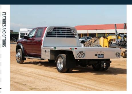
NOTABLE OPTIONS INCLUDE: 3/16" Heavy-Duty Deck; 30K B&W Hitch with Turnover Ball (required for 5th Wheel capability); Cargo Light; Drop-In or Fold-Down Side Rails; Gooseneck Trough; Wood, Rumber or Blackwood Flooring;
